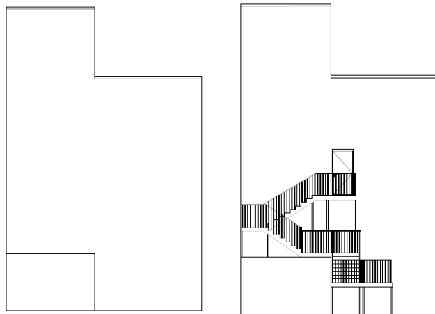
Existing (left) and proposed (right) east elevation plans
