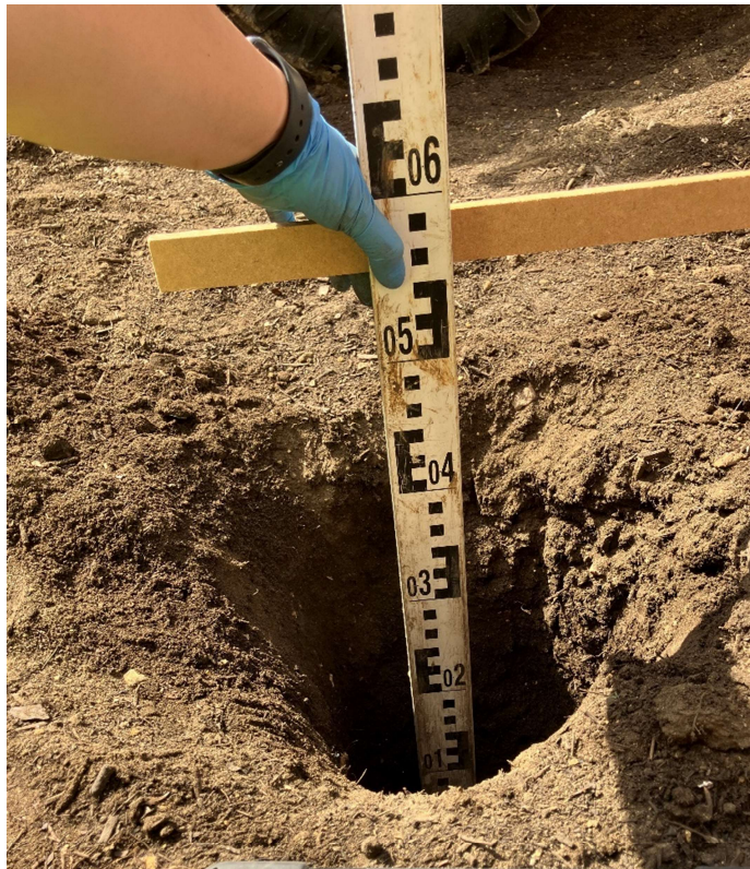
Figure 4: HP2 with 450mm of topsoil noted.
