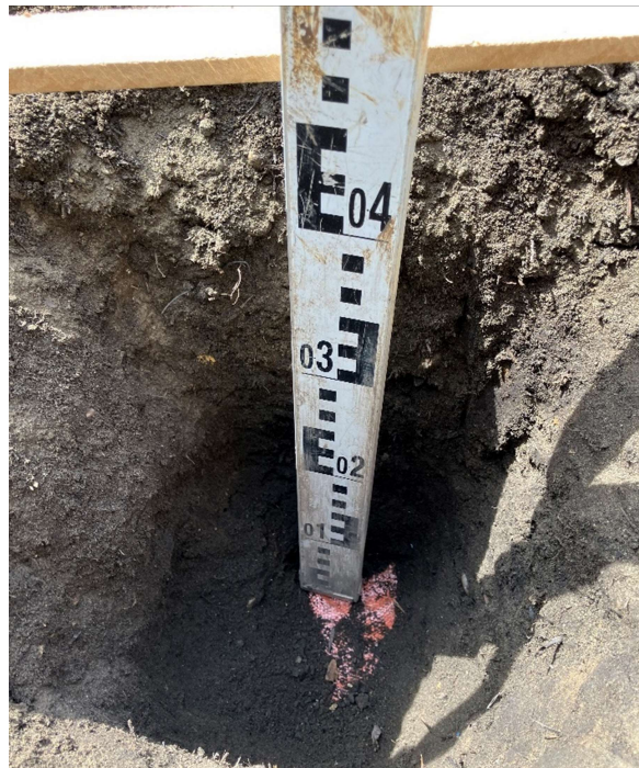
Figure 8: HP3 noted with orange marker membrane at base
