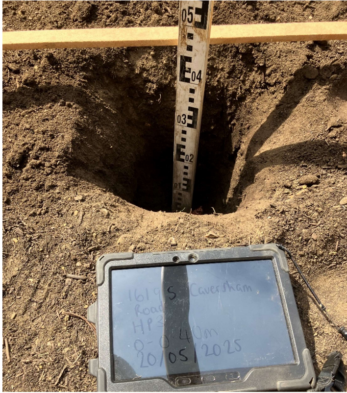
Figure 7: HP3 noted with 400mm of soil. Final soil levels will be approximately 470mm once topped up to finishing level.
