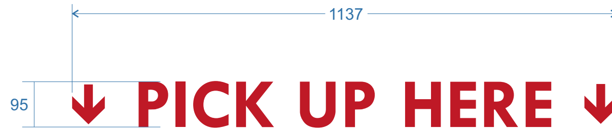
Scale 1:8 installed to bulkhead centrally above collection point
