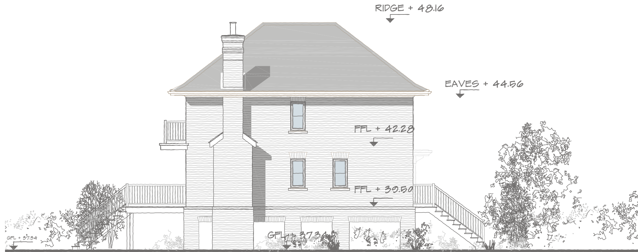
SIDE ( EAST ) ELEVATION
