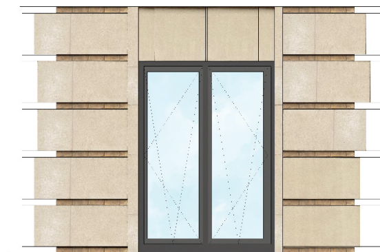
New Ground Floor Tilt and Turn windows
