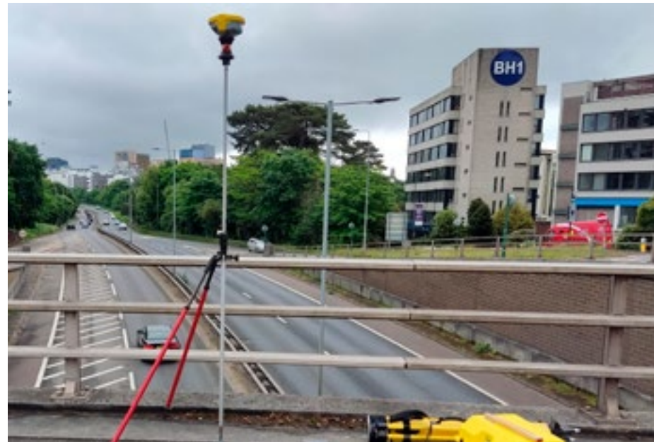
7: Field survey being carried out, GNSS receiver
