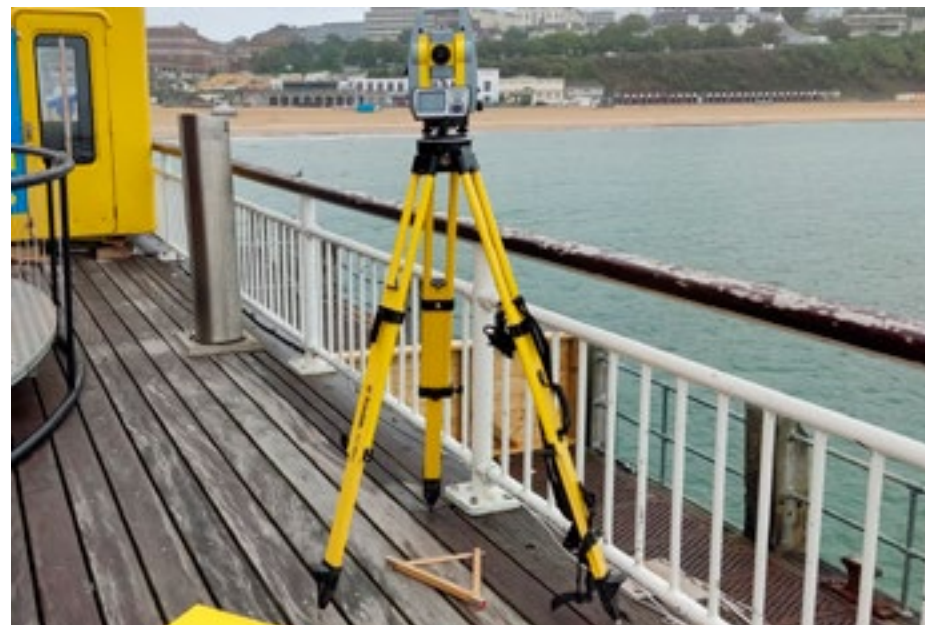
8: Field survey being carried out, total station
