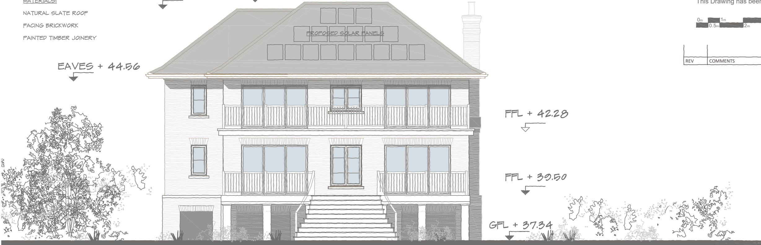
REAR ( SOUTH ) ELEVATION - FACING RIVER
