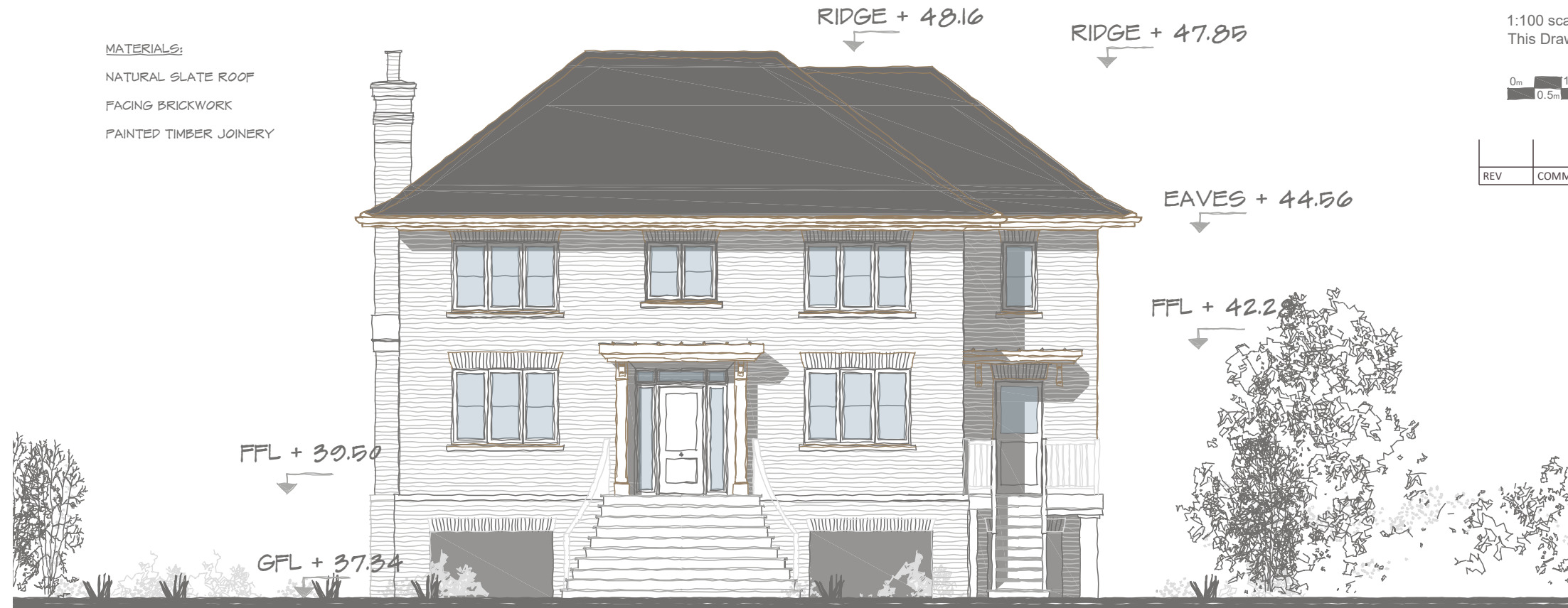
FRONT ( NORTH ) ELEVATION - FACING ROAD
