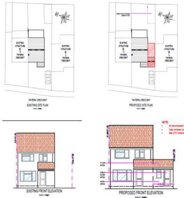
Figure 2 - Existing and proposed site plan and front elevations
