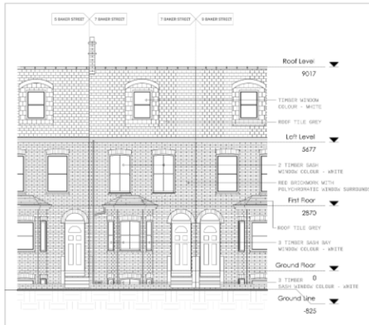
FRONT ELEVATION EXISTING
