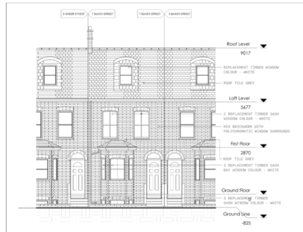
FRONT ELEVATION PROPOSED REPLACEMENT WINDOWS
