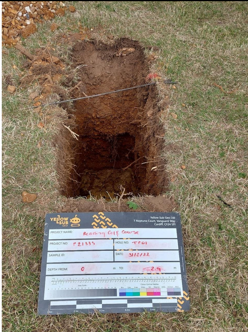
TP01 trial pit
