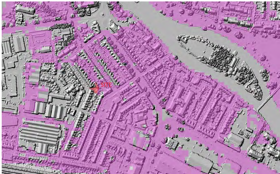
Figure 4.3 – Modelled Flood Zone 1.0% Probability with CC Allowance
