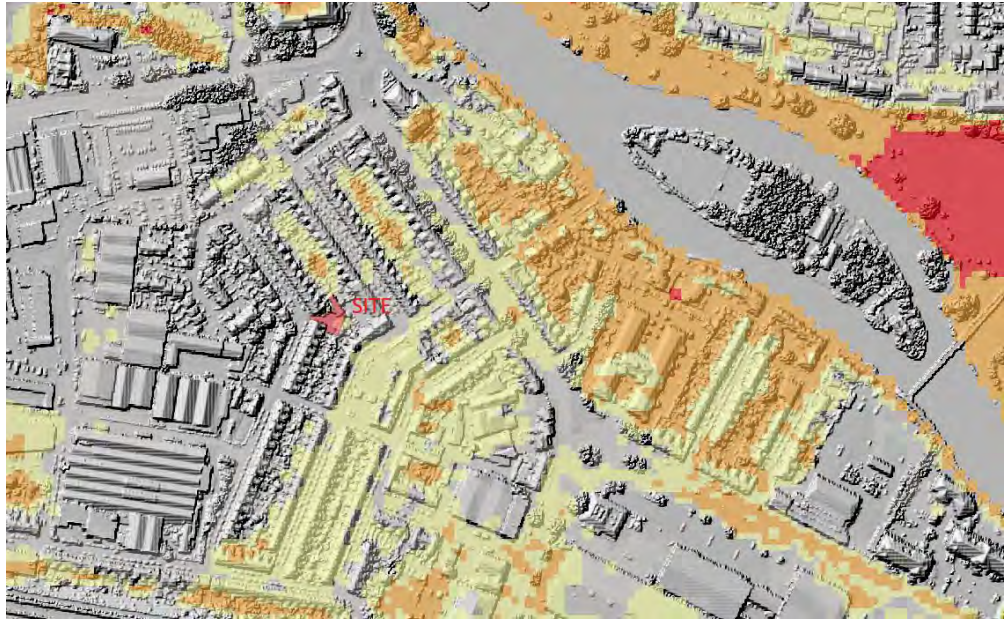
Figure 5.1 – Flood Hazard Map for 1.0% AEP +CC
