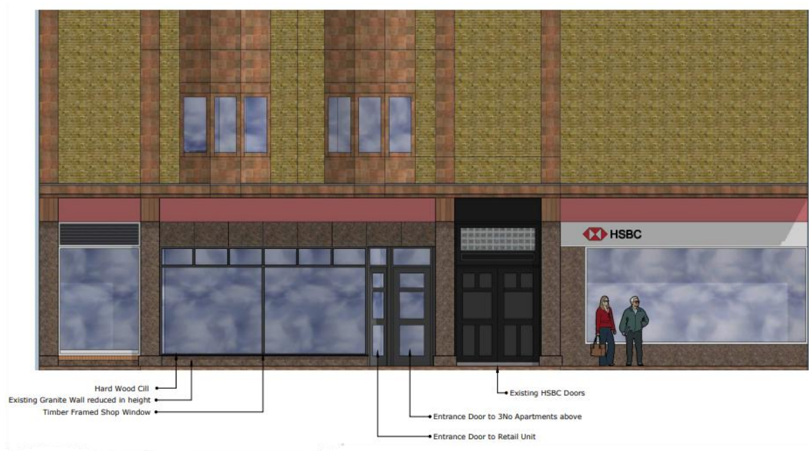
Fig. 12. The revised shopfront with timber frame, clerestory lights, chamfered entrance to the shop and separate access to the flats above. Source: Ian Benbow
