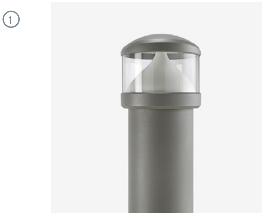
Reference/Product: B01/DW Windsor Kirium Pro 200 Bollard Description: 1m tall Lighting bollard with high vandal and impact resistance and low glare shielded optic. 20W, 2100lm, 2700K, narrow asymmetric optic.
