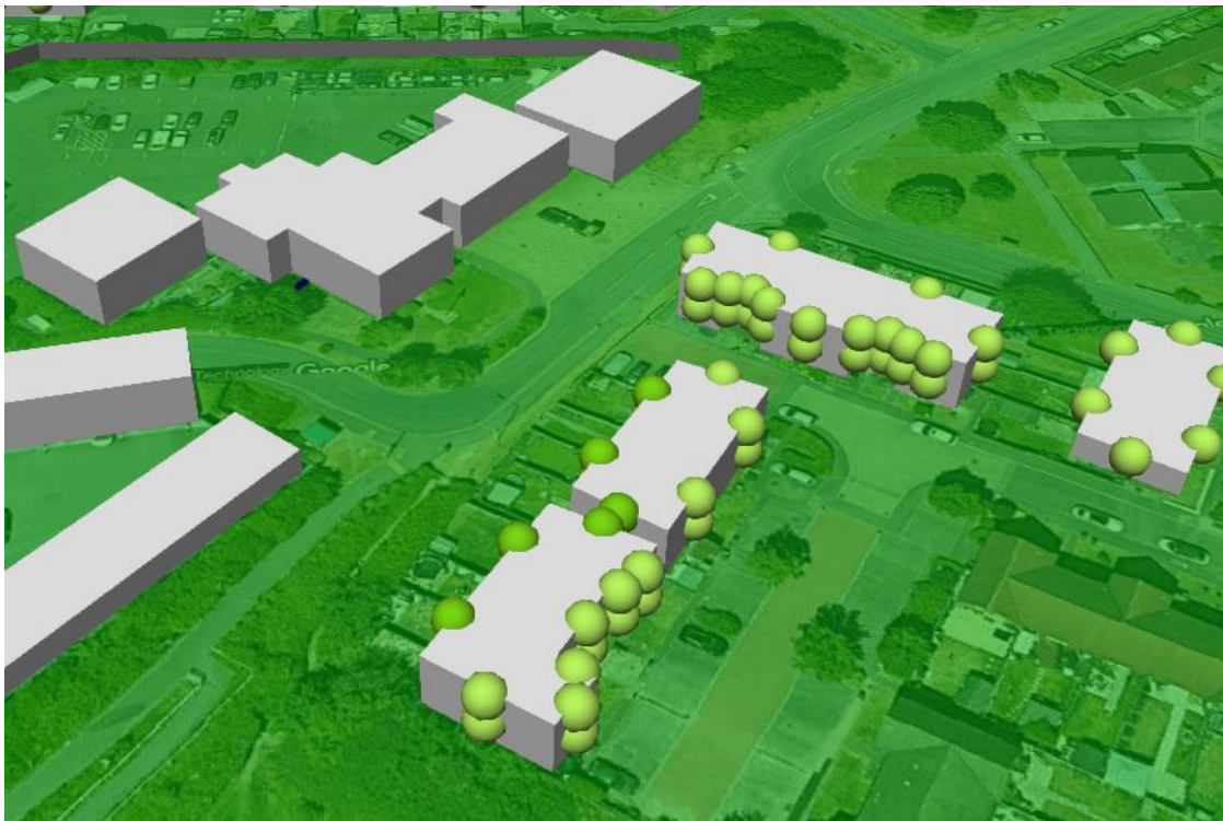
Figure 5.2: 3D Acoustic model with noise sources
