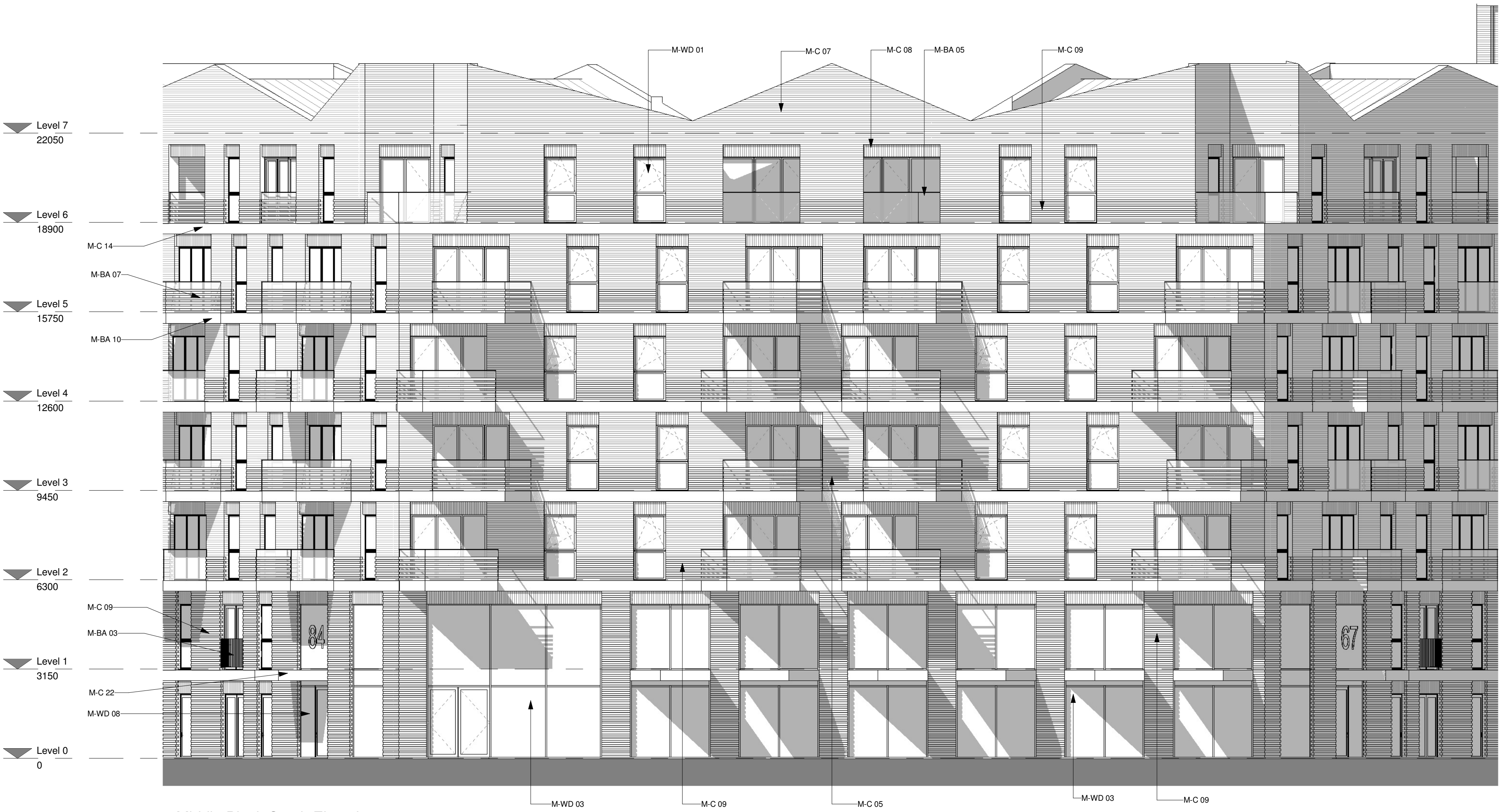
Middle Block South Elevation 1 : 100
