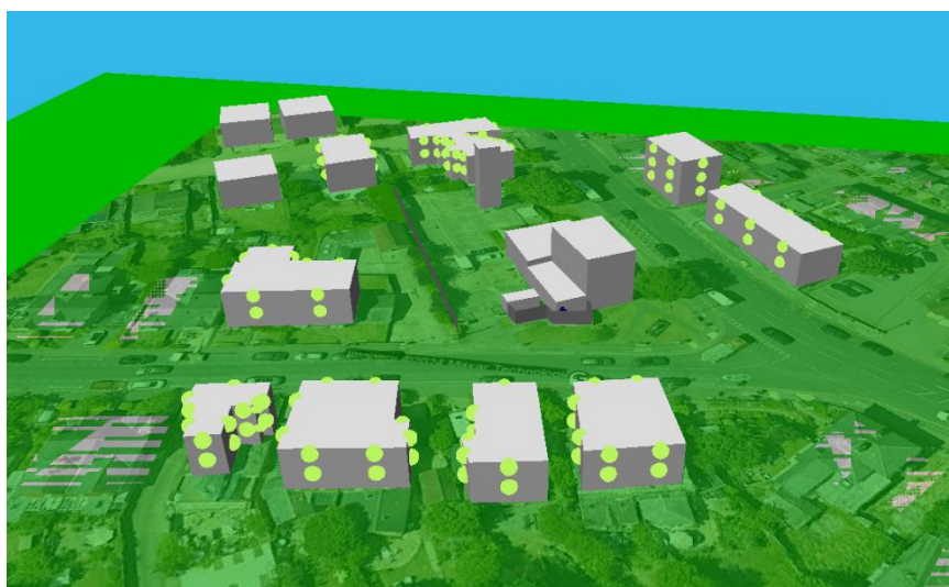
Figure 5.2: 3D Acoustic model with noise sources
