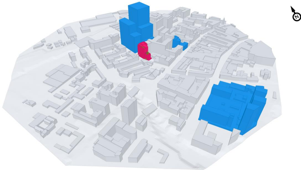
Figure 16: Proposed Development (pink) with Cumulative Surrounding Buildings (blue) 3D model used for Computational Fluid Dynamic simulations (view from the south-west)
