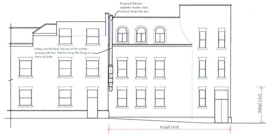
Proposed Side Elevation - Part - (viewed from South Street)
