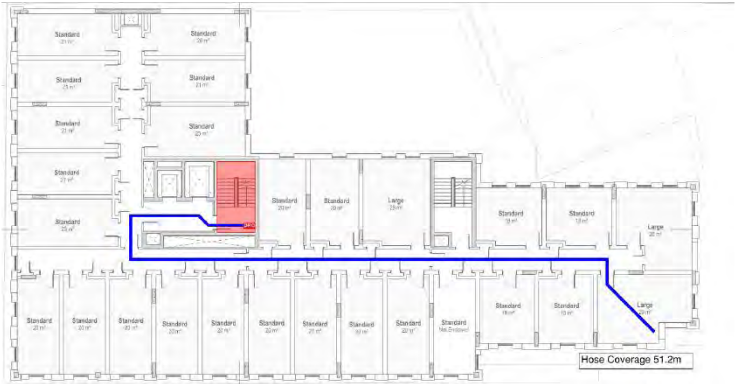
Fire service site plan (source: Orion Fire)
