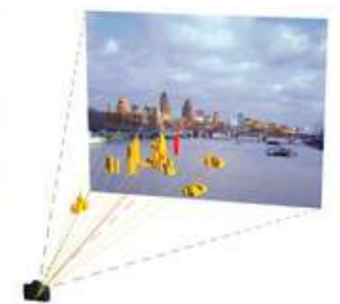
17: The camera matched background plate with an example of a proposed scheme included in red
