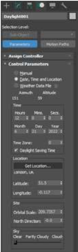
22: Screenshot of environment information (time, date and year) entered to locate the sun correctly (see Section 7).
