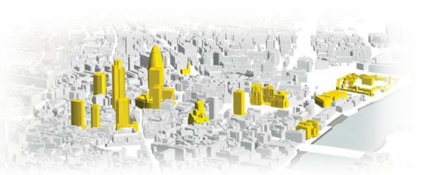
14: Selected GPS located models (yellow) from Cityscape's database, situated on Cityscape's London digital terrain model
