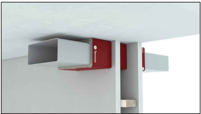
Fig 1: Where ductwork passes through 30 minute fire compartment walls within flat, duct to be fire wrapped
