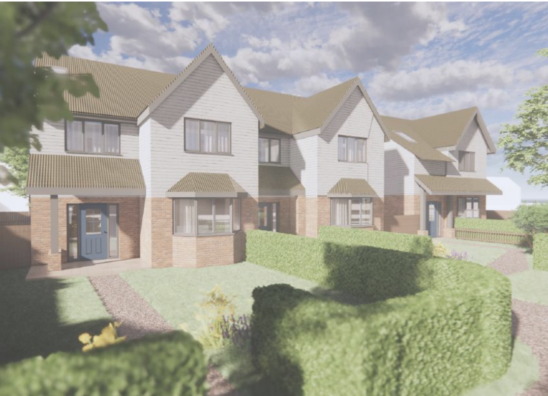
Light grey weatherboarding, with asphalt grey fascia boarding and painted window frames
