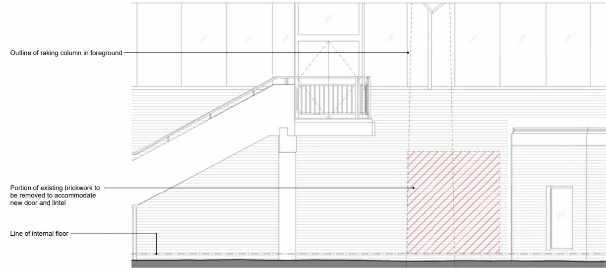
3 / GET-IN - EXISTING & DEMOLITION ELEVATION
