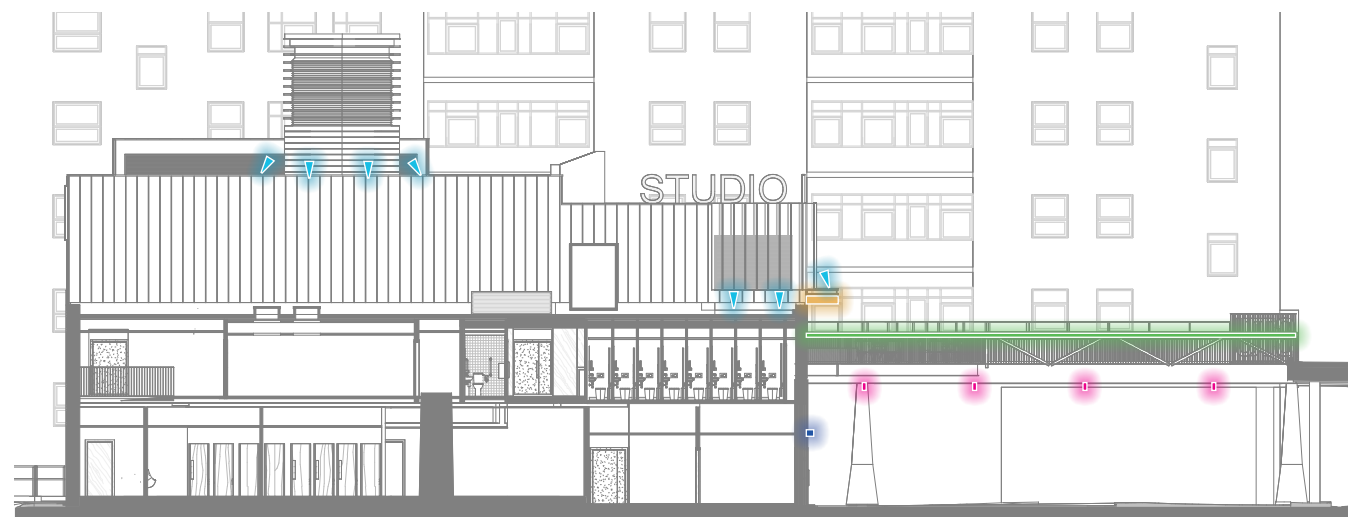
South Elevation - Proposed External Lighting
