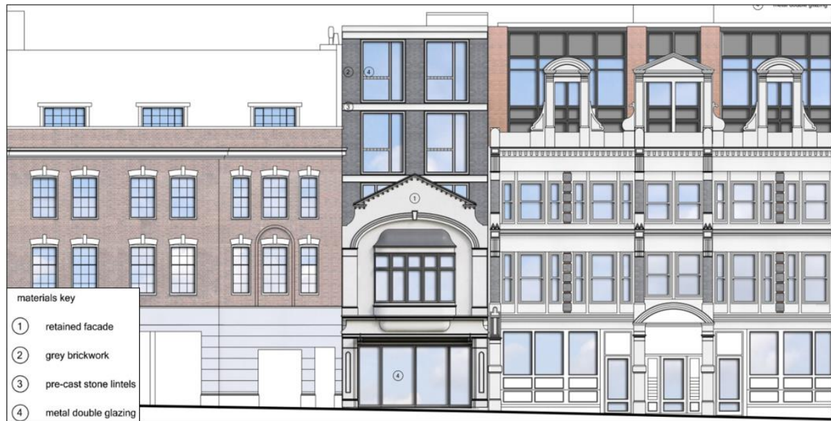
Fig. 9: Architect's drawing of the proposed street elevation of No. 7 Blagrove Street and surrounding buildings, incorporating the new building behind the retained frontage (bad-studio architects).
