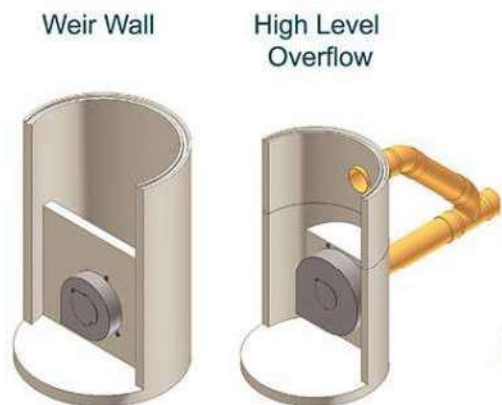
Figure 2-8: Typical vortex control device with overflow allowances
