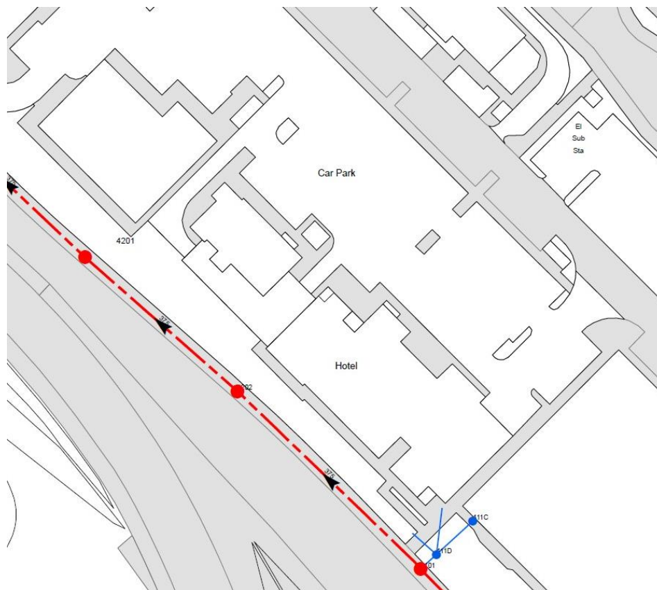
Figure 2: Thames Water Sewer Records
