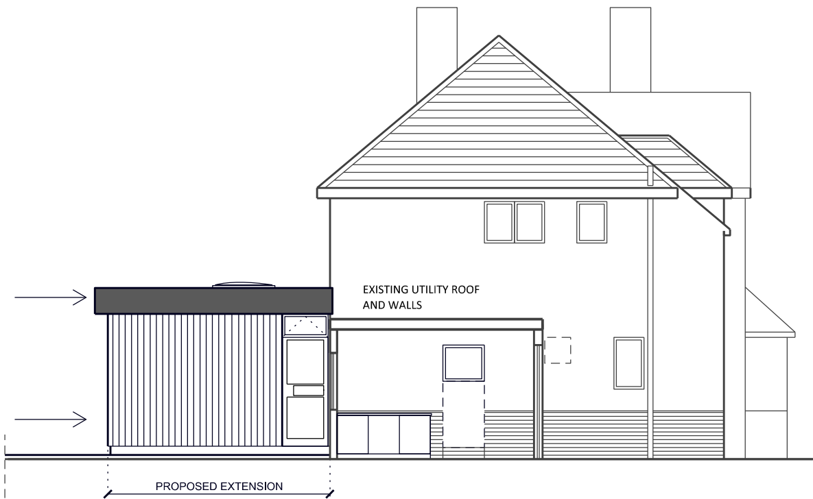
SIDE (SOUTH-EAST) ELEVATION
