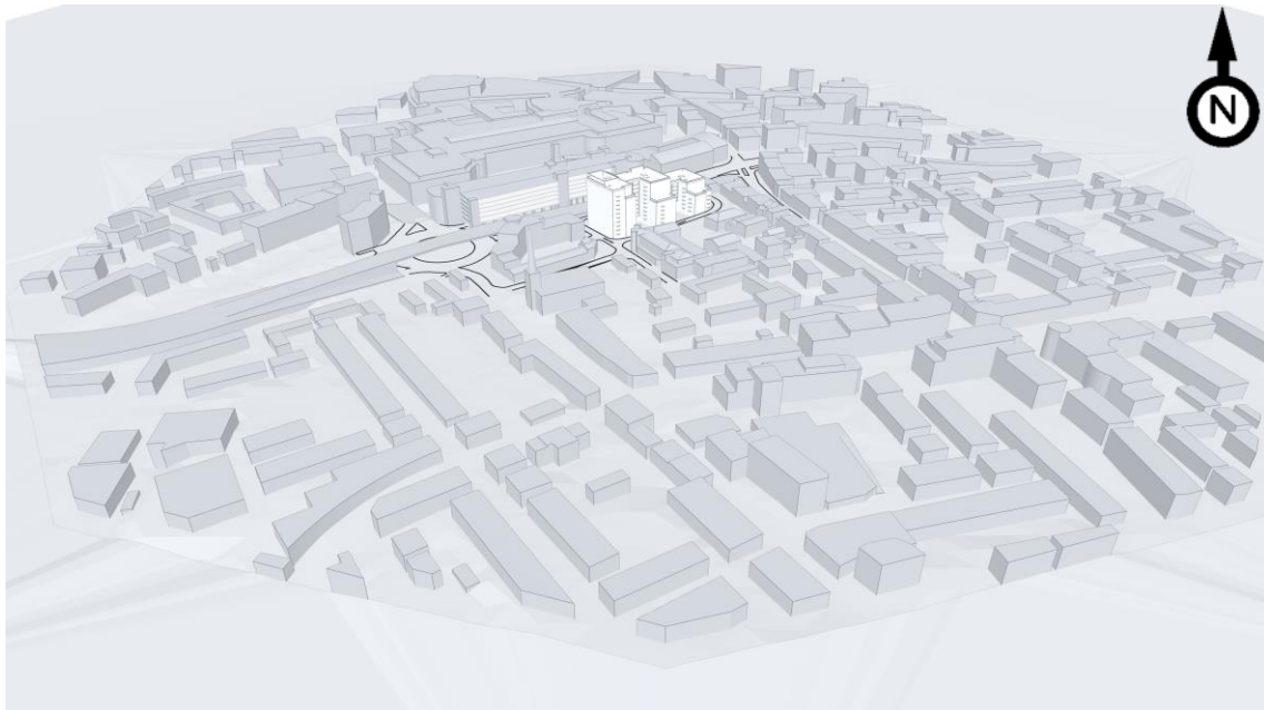
Figure 30 – Existing Site with Existing Surrounding Buildings 3D model used for Computational Fluid Dynamic simulations (view from the south)
