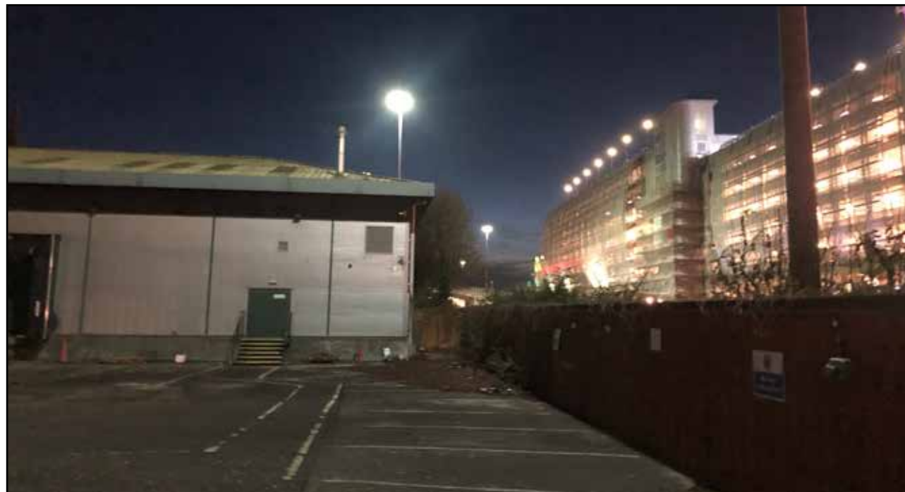
Figure 5.63 Showing loading bays with Site lighting off, looking south-west. Luminaires mounted on approx. 6m & 30m along Mill Lane/MSCP visible. Captured at approximate position of Survey Location A6.
