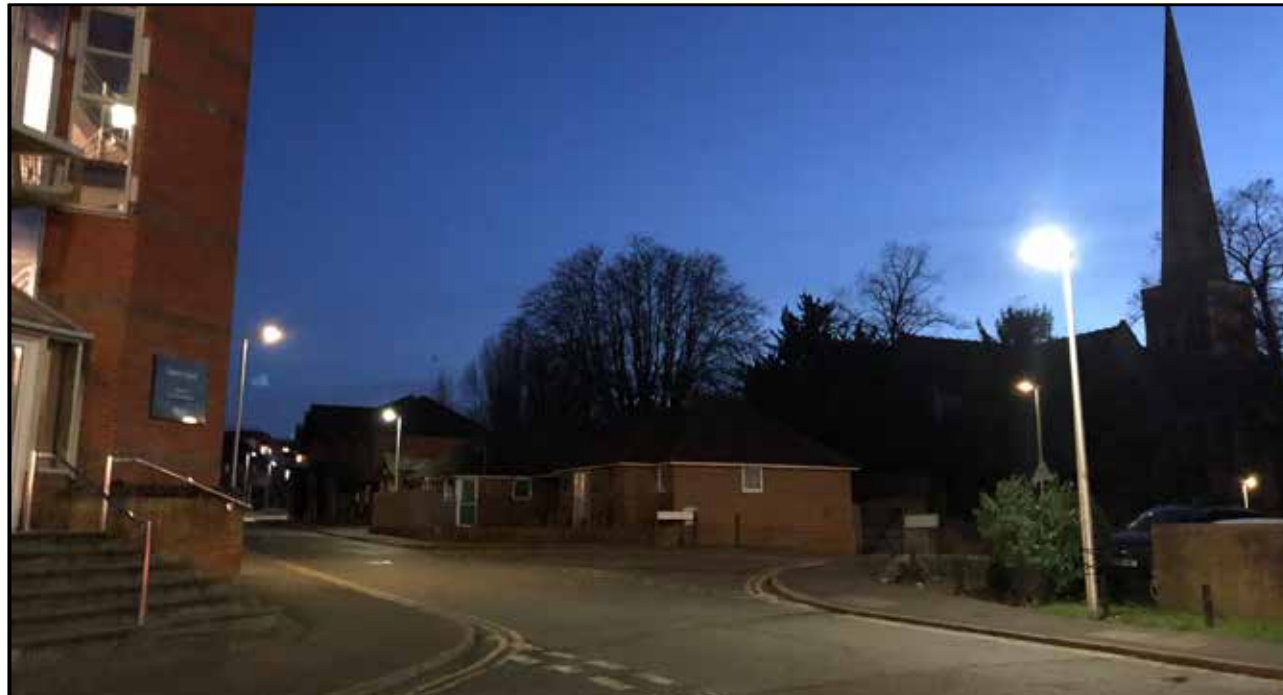
Figure 5.16 Showing LED luminaires mounted on approximately 6 metre high columns along Church Street, facing south-west. Townsend House on left of image. Captured at approximate position of Survey Location R1.
