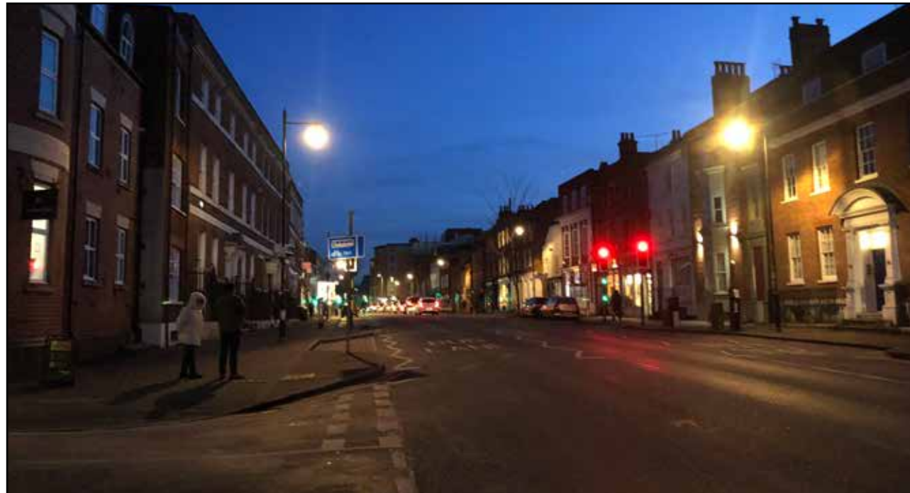
Figure 5.65 Showing luminaires mounted on approximately 6 metre high columns along London Street, looking north. Captured at approximate position of Survey Location A14.
