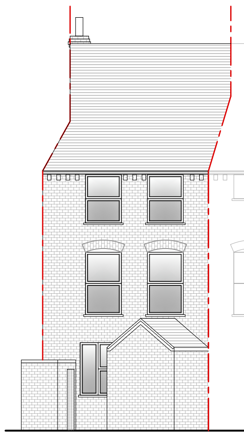
7 Existing Rear Elevation
