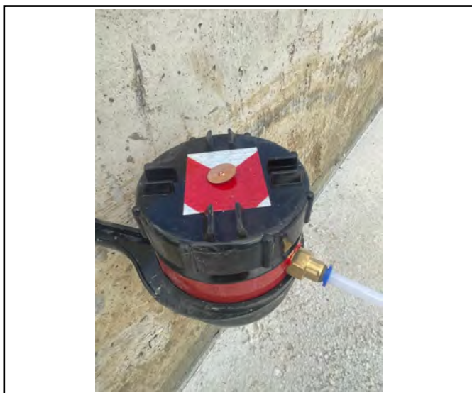
Ground gas monitor fixed.
