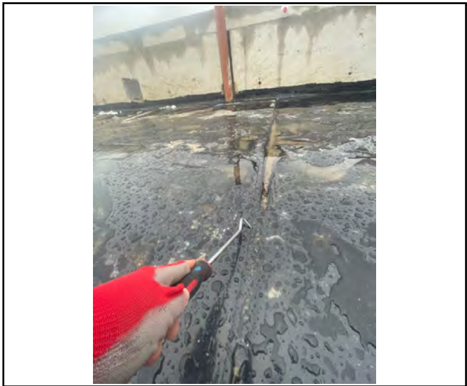
Pick&probe testing to welded lap joint.
