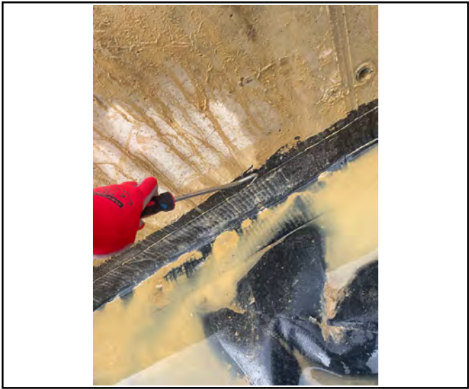
Pick&probe testing to retrofit detailing.
