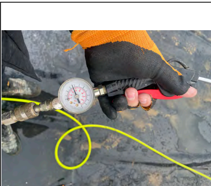
Airlance integrity testing to welded lap joint.
