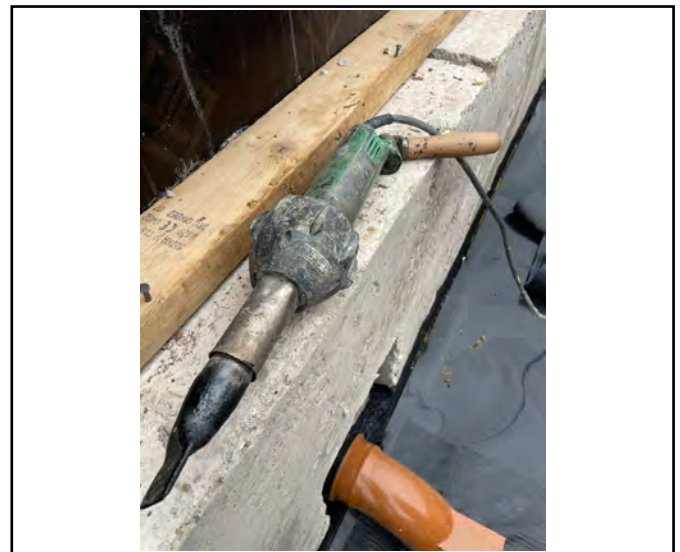
Photograph above shows a hot air leister used onsite.
