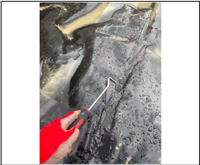
Pick&probe testing to welded lap joint.
