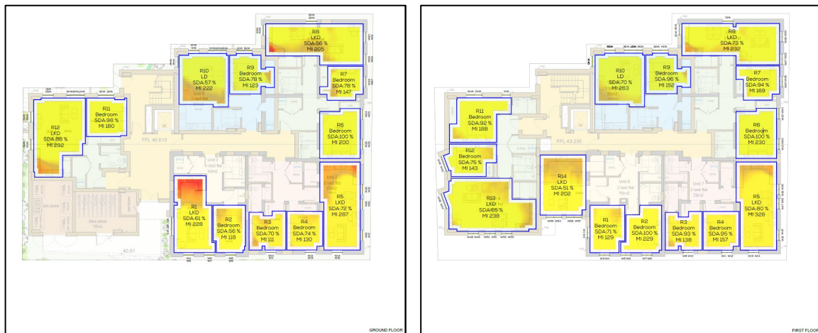
Figure 05 & 06 – Ground & First Floor Spatial Daylight Autonomy Analysis
