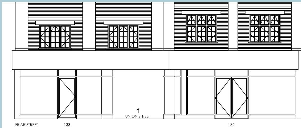
Figure 10: Existing Shopfront Elevation (© THP)
