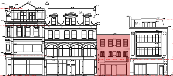
Existing Friar Street elevation. Extent of re-construction to no.146 highlighted in red.
