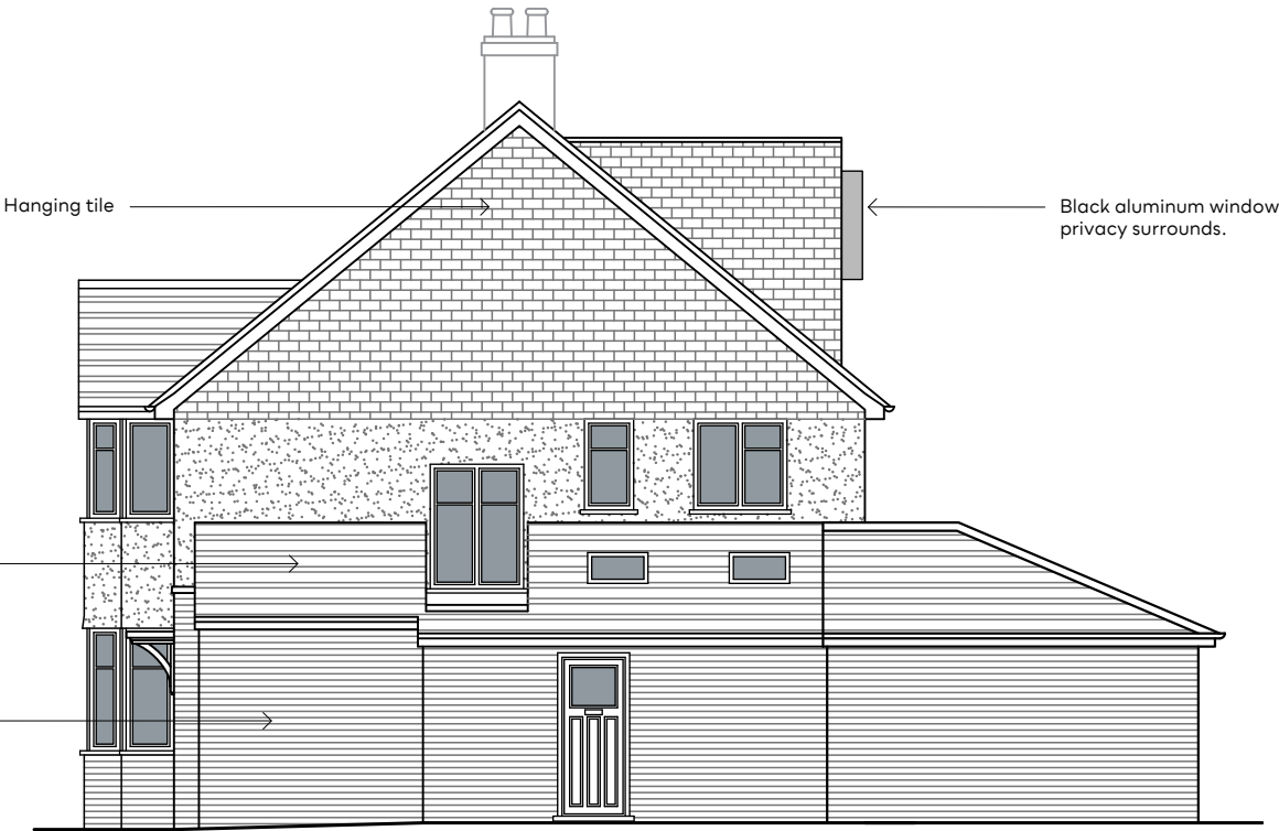
SIDE ELEVATION (NORTH FACING)
