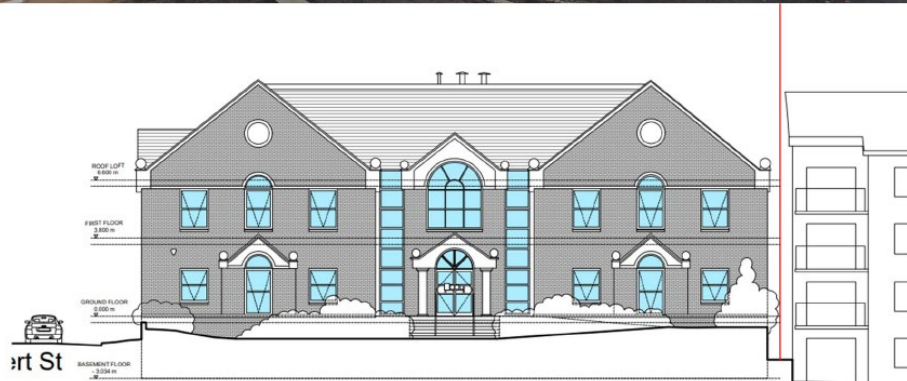
Image 1: Brick Banding missing from Approved Existing elevation
