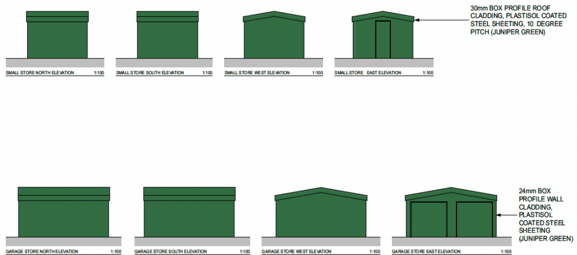
Figure 2: The proposed storage buildings
