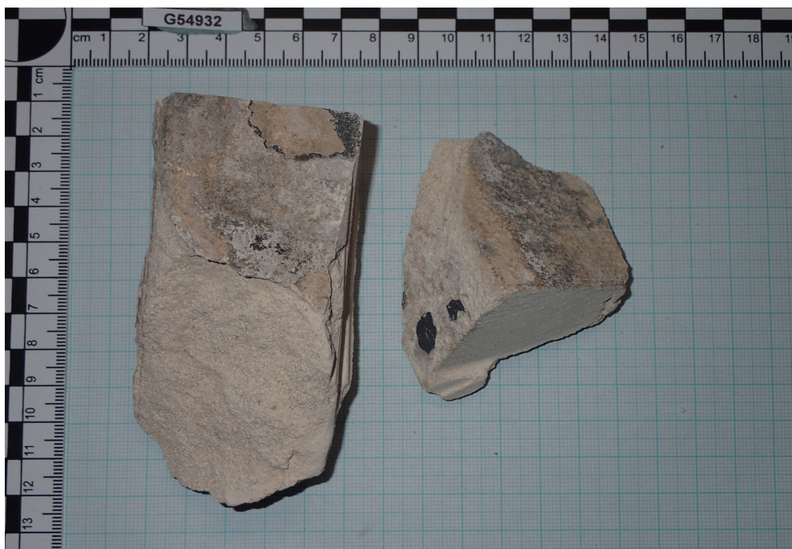
G54932. View of sample received exhibiting exposed and broken / sawn surfaces.
