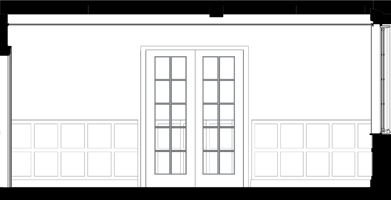
AS PROPOSED SECTION THROUGH THE GROUND FLOOR FRONT ROOM SHOWING THE NEW PARTITION IN ELEVATION. THE REVERSE SIDE WOULD HAVE THE SAME APPEARANCE.
