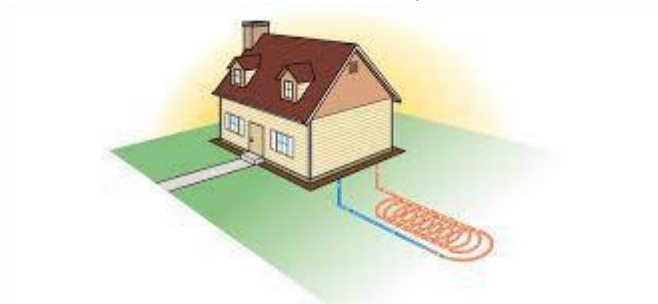
Figure 8: Ground Source Heat Pump
