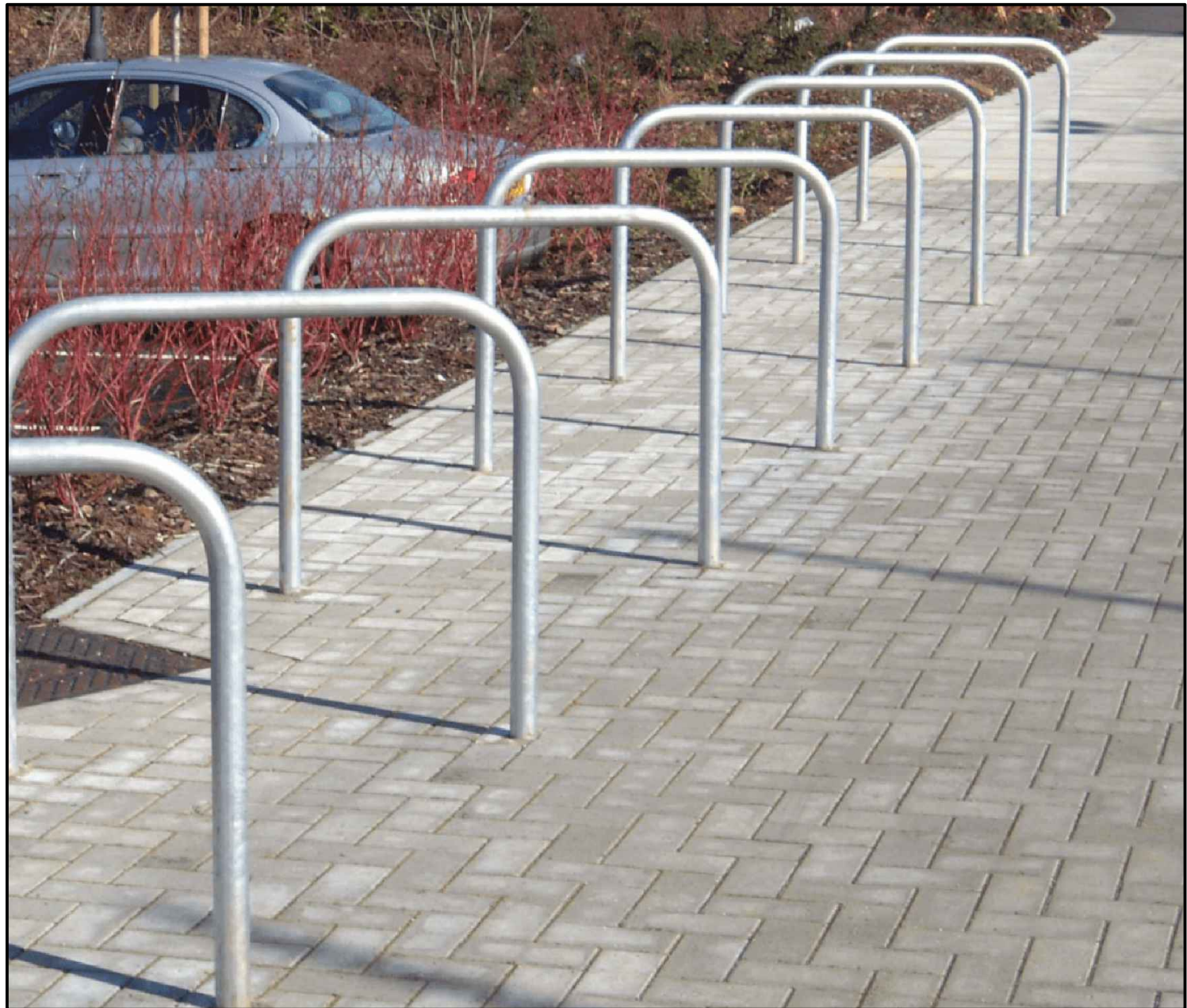
D4 CS - SHEFFIELD CYCLE STAND ; SUPPLIER: CYCLEHOOP; FIXING: ROOT FIXED SCALE NTS
