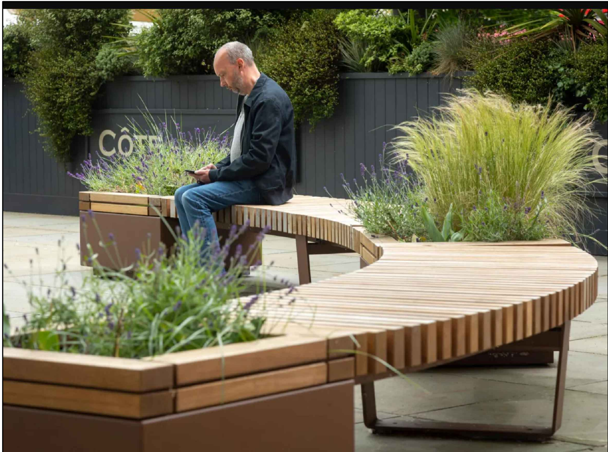
D2 B2 - LONG SEAT;TIMBER SLATS AND GALVANISED POWDER COATED STEEL LEGS, SUPPLIER: FURNITUBES SCALE NTS
