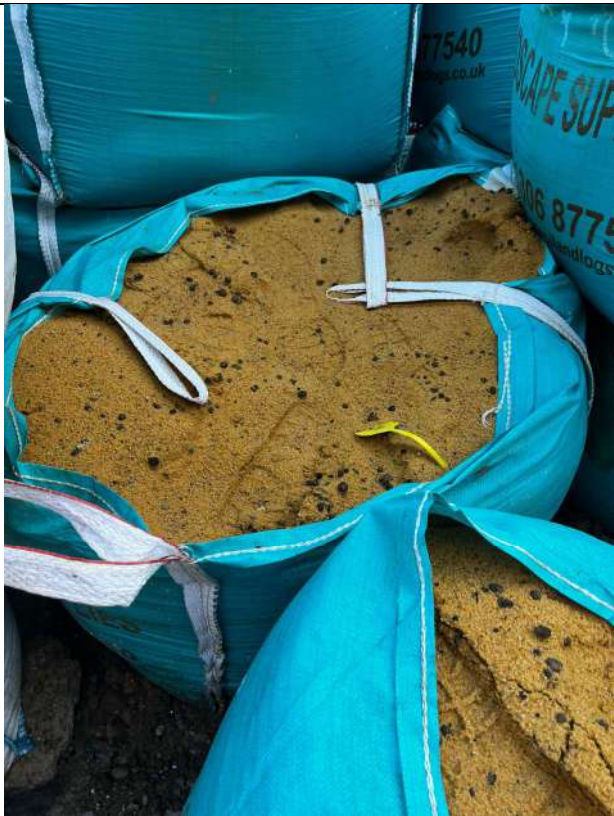
Photograph 02 Bulk bag of subsoil delivered to the site.
