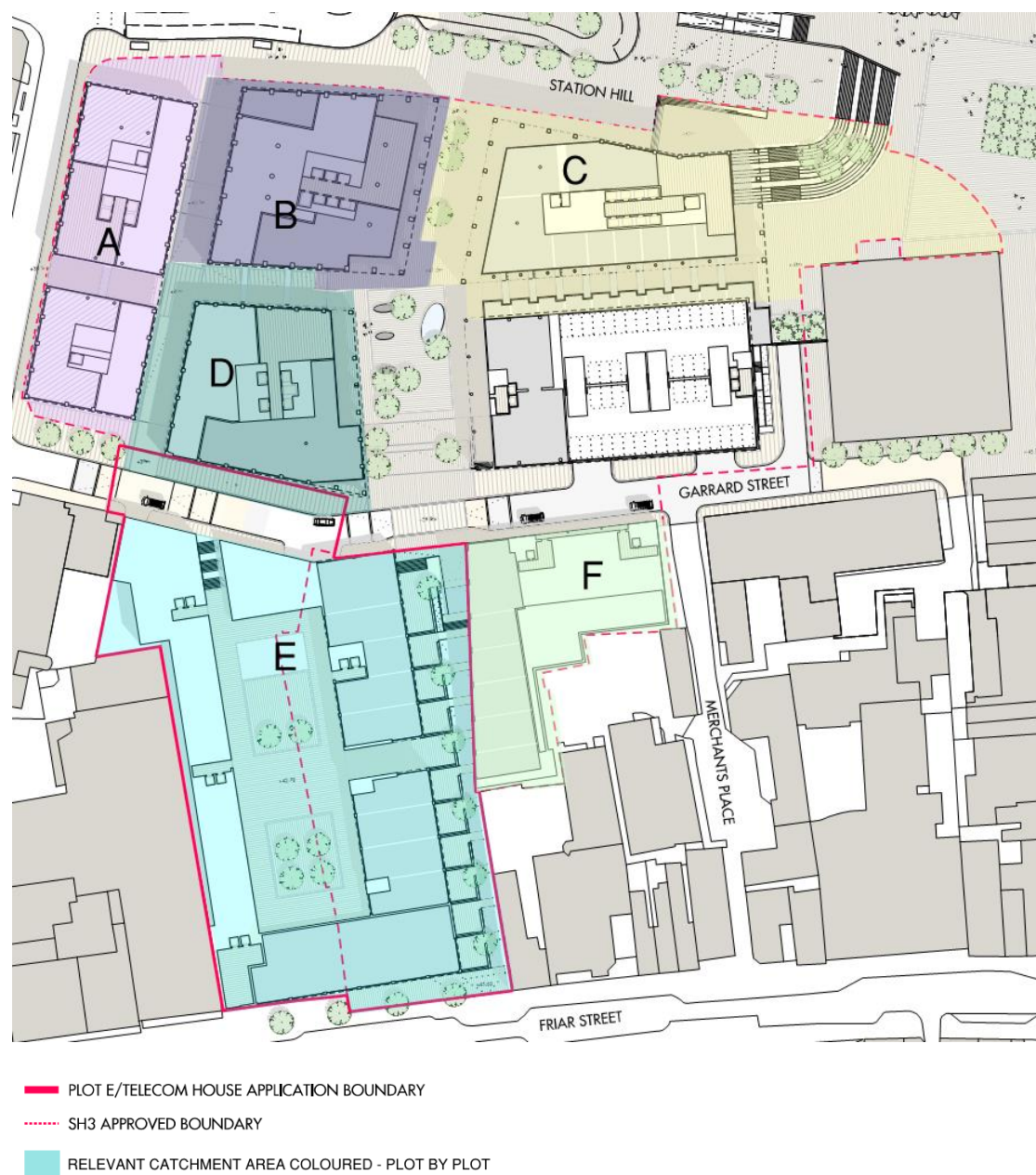
Figure 1. Drainage Catchment Areas
