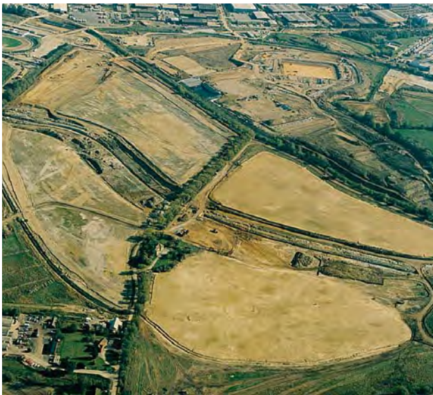
The formation of development platforms in 1996 above flood levels
