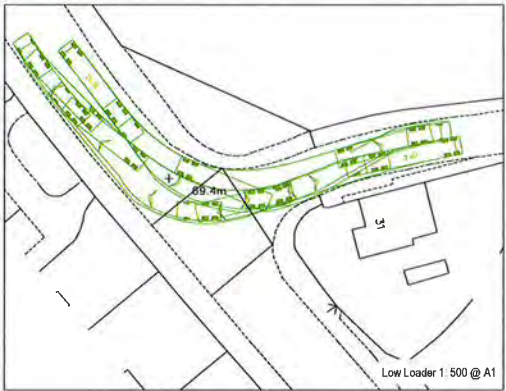
SHINFIELD ROAD SWEEP PATH ANALYSIS : SITE ENTRANCE & EXIT
