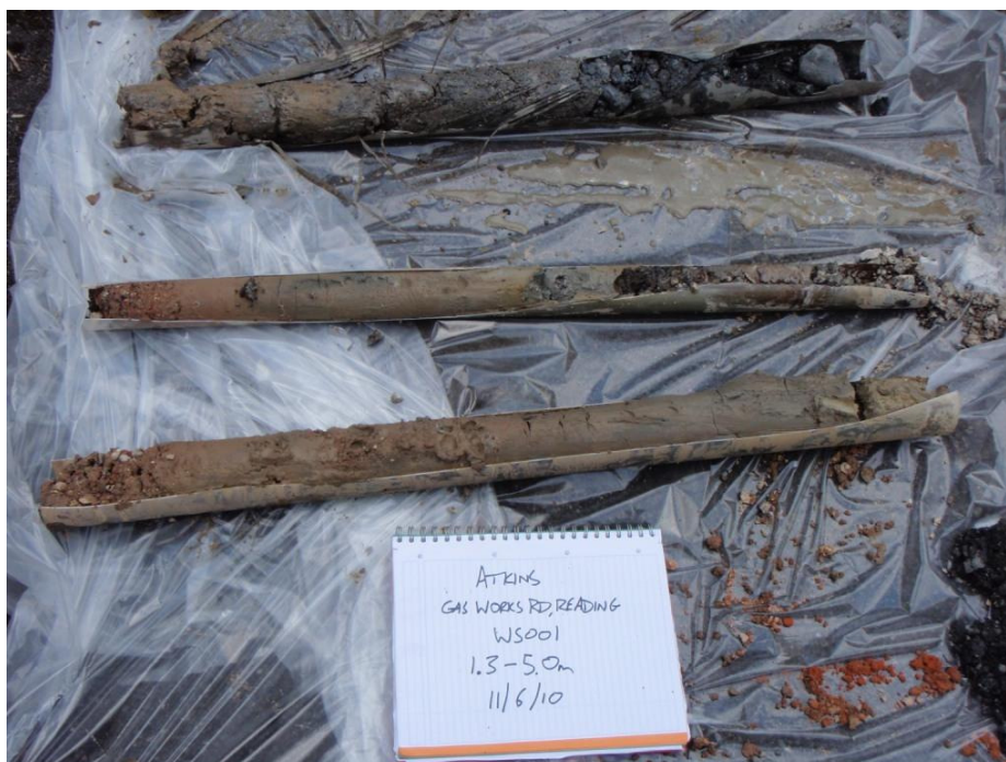
Photo 4: Window sample core from WS001. Note black hydrocarbon staining, indicating previous remediation in this area was not fully completed.
