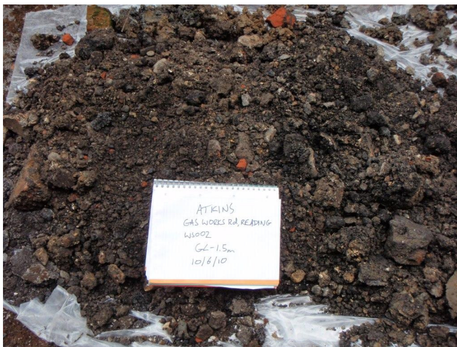
Photo 2: Typical Made Ground encountered at the site.
