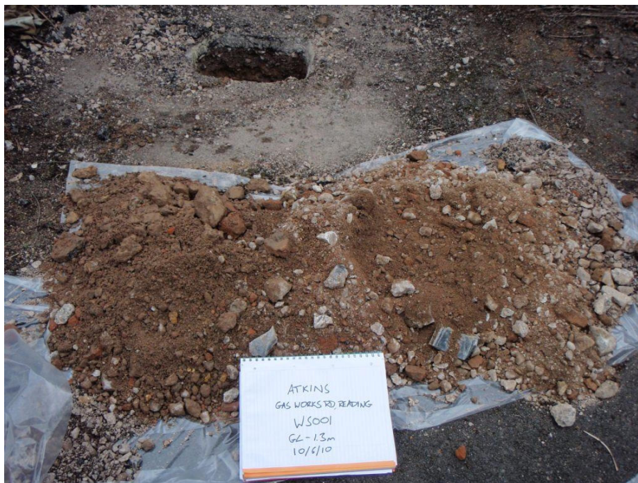
Photo 3: Fill material encountered in WS001 (in previously remediated area).
