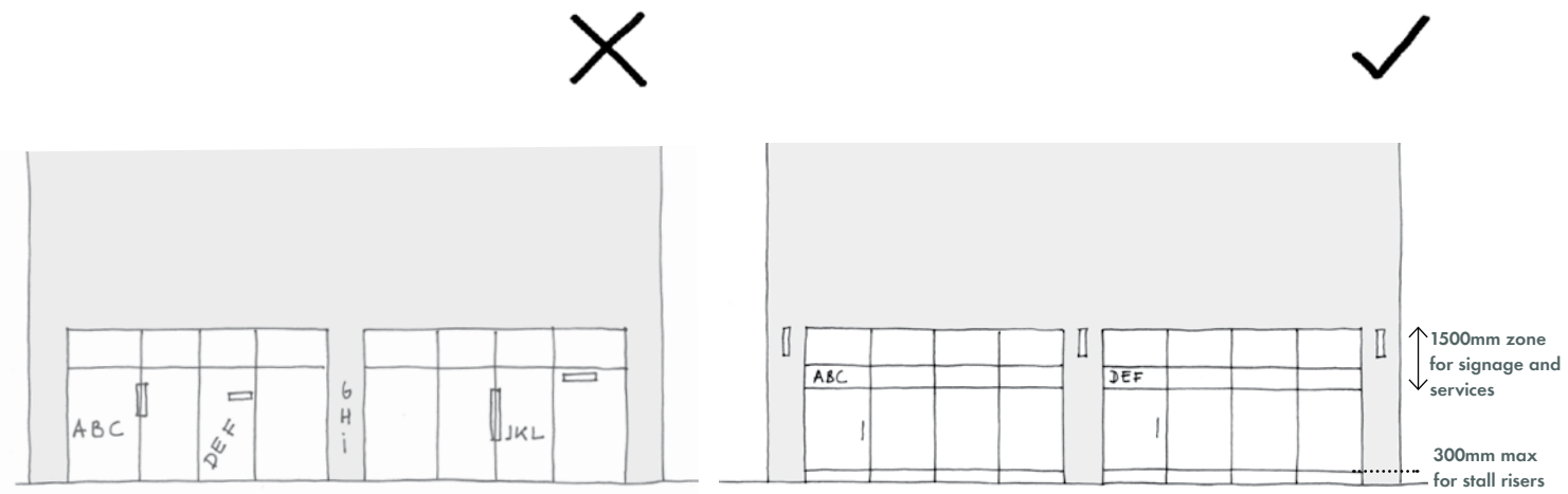
Figure 16: Retail facades - Shop signage and stall risers
